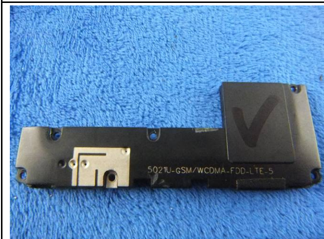
GSM/PCS/UMTS-FDD Antenna View
