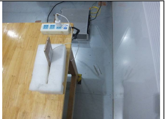
Conducted Emissions Test Setup Side View
