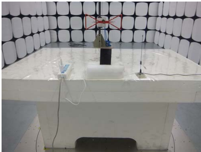
Radiated Spurious Emissions Test Setup Below 1GHz
