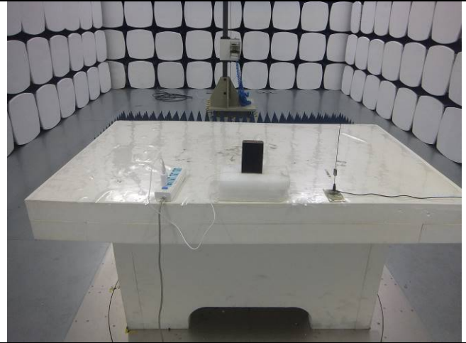
Radiated Spurious Emissions Test Setup Above 1GHz
