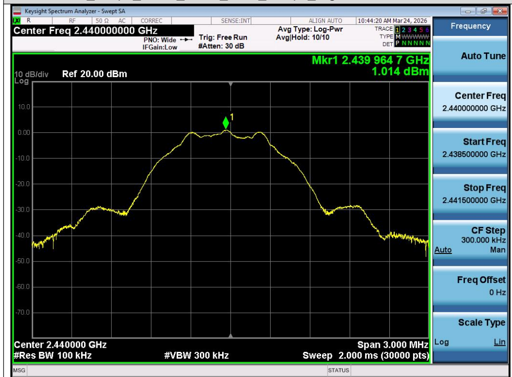
Test Graph LE1M ANT1 2440 1Mbps Reference Level
