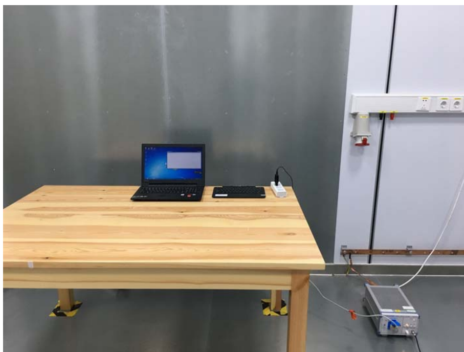
Fig. 4 Power line conducted emission setup photo
