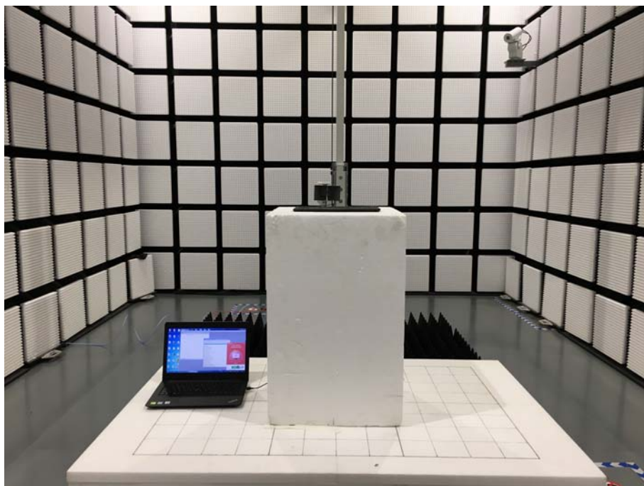
Fig. 3 Radiated emission setup photo(Above 1GHz)
