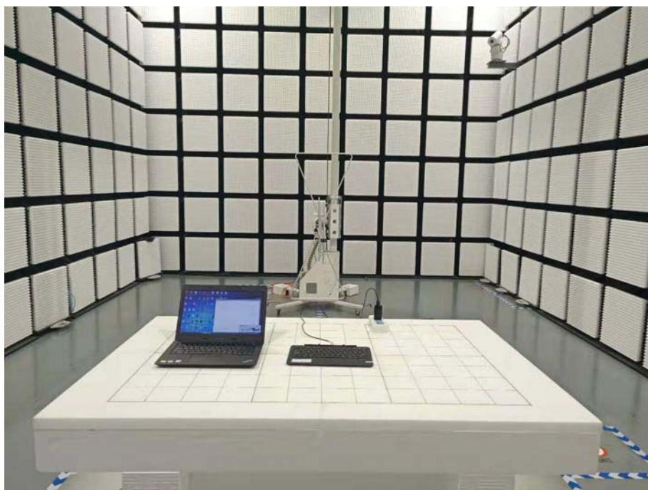
Fig. 2 Radiated emission setup photo(30MHz-1GHz)
