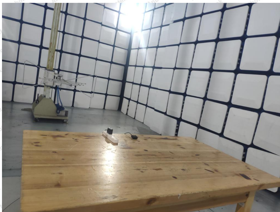
Photo of Radiation Emission Test
