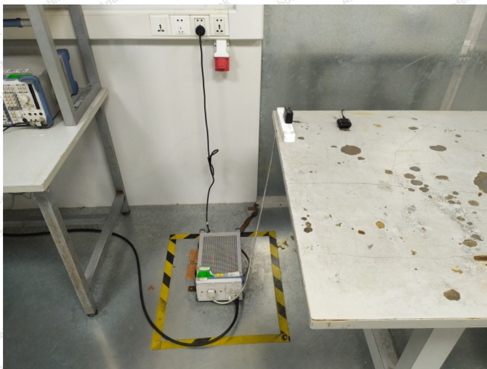
Photo of Conducted Emission Measurement
