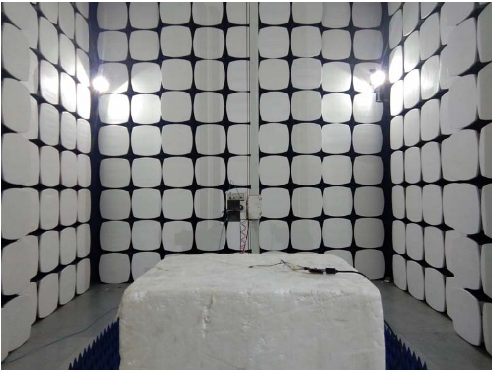
Radiated Setup photo (Above 1G)
