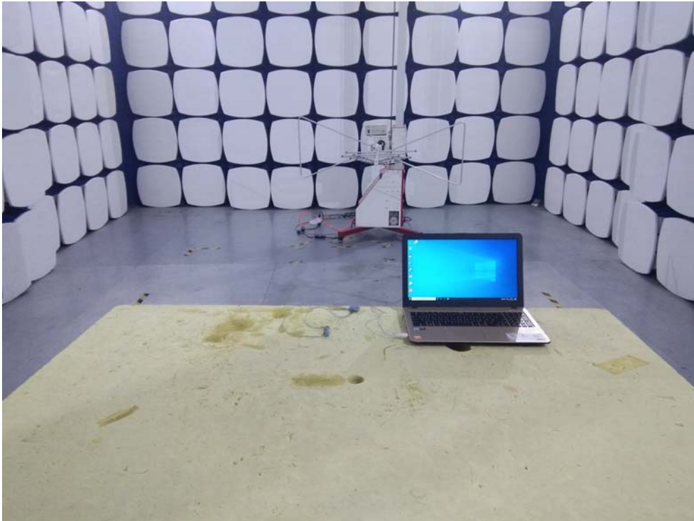
Radiated Setup photo (Below 1G)
