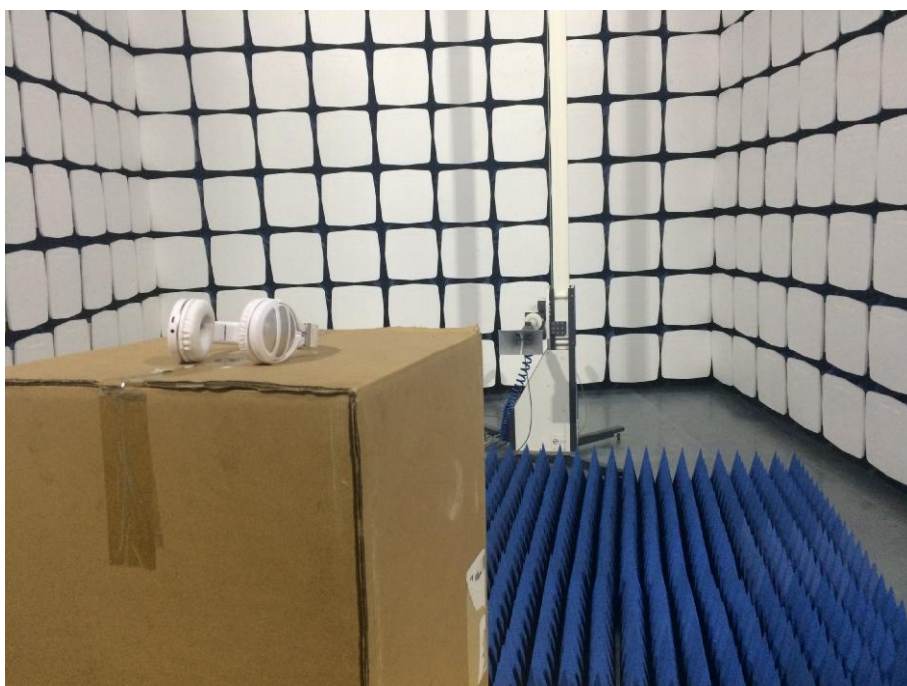
Radiated Emission test view (Above 1GHz)
