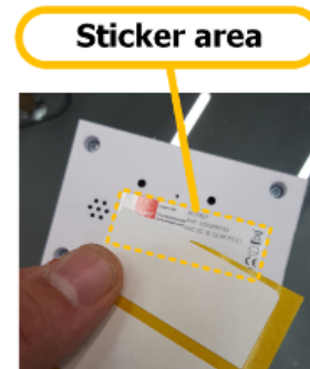
3. Apply the double-sided tape to the reader. Make sure to stay within the serial sticker area!
