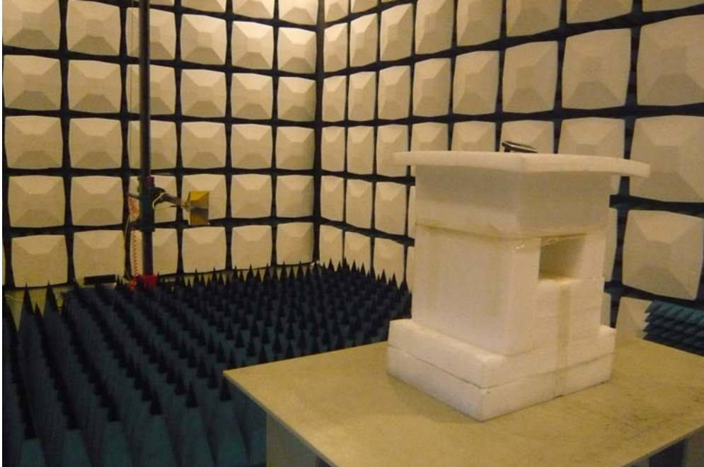
Radiated Emission View (Above 1GHz)
