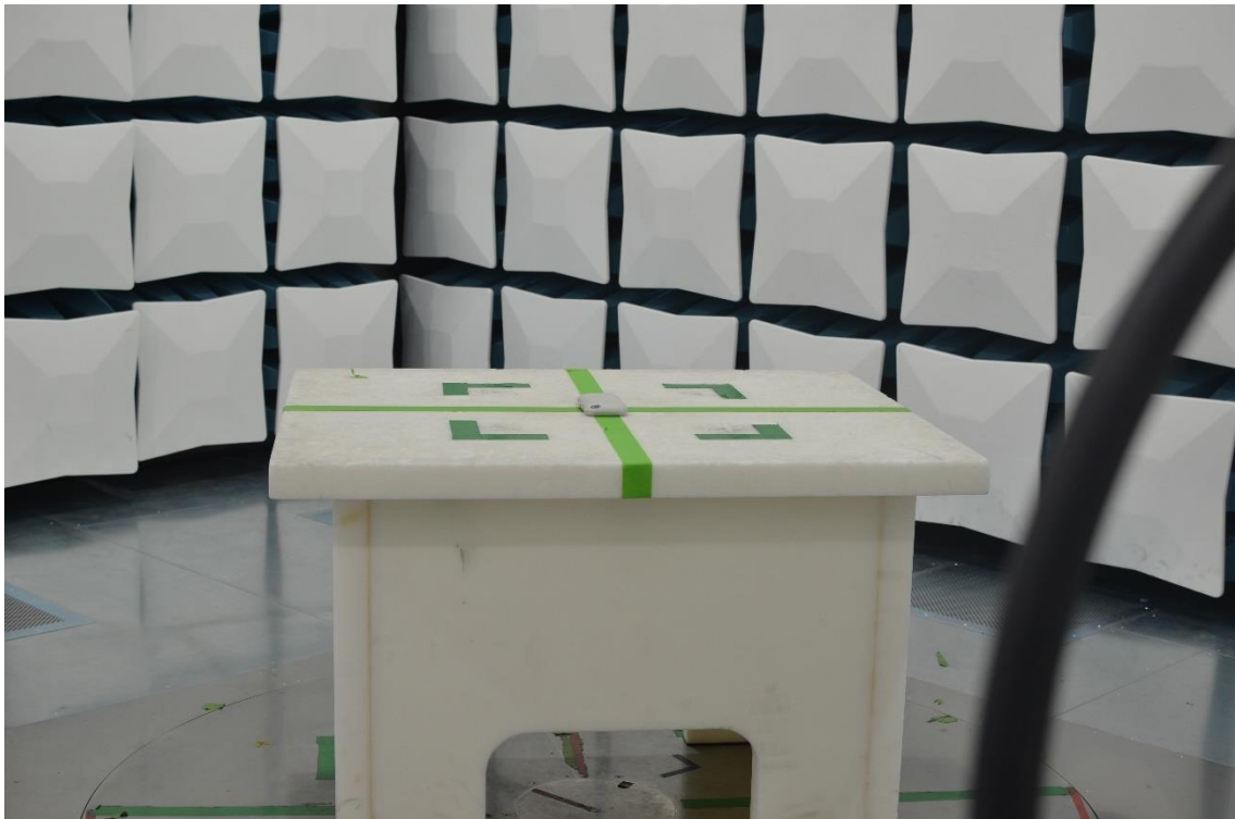
Figure 13: 9kHz-30MHz Test Setup (Front View)
