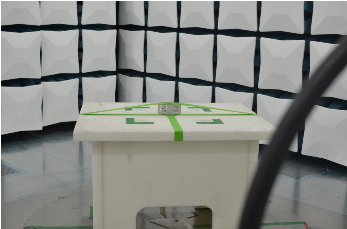
Figure 14: 9kHz-30MHz Test Setup (Front View)
