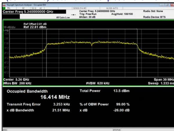
(802.11 n20) 99% Bandwidth plot on channel 48
