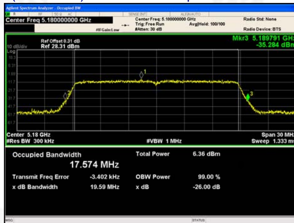
(802.11 n20) 26dB Bandwidth plot on channel 36
