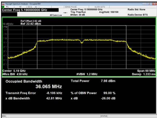
(802.11 n40) 26dB Bandwidth plot on channel 46
