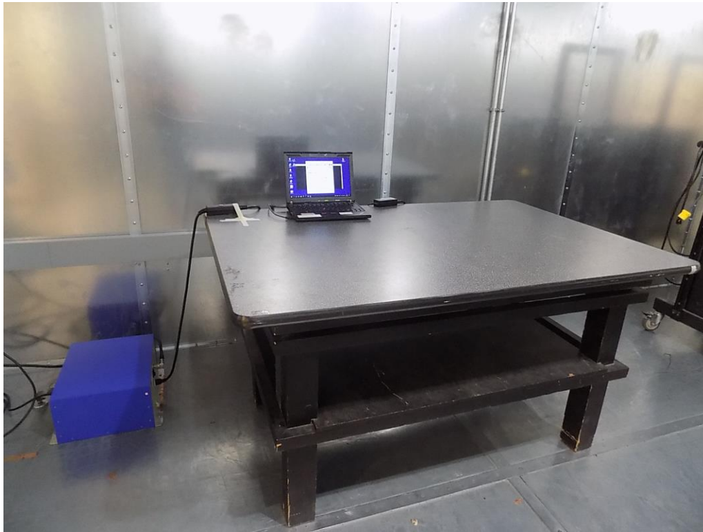
Figure 12 - Conducted Emissions Test Setup - Front
