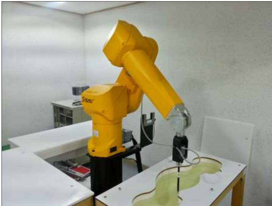
Photograph of the SAR measurement System
