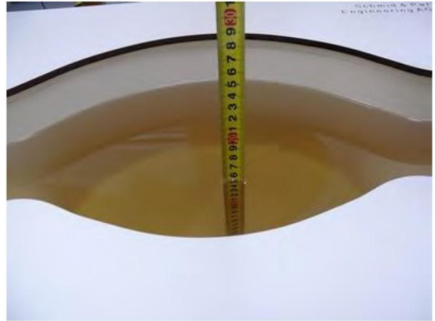
Liquid depth in the body phantom (835MHz)
