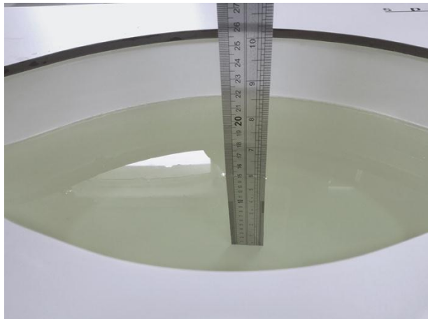
Liquid depth in the body phantom (2450MHz)
