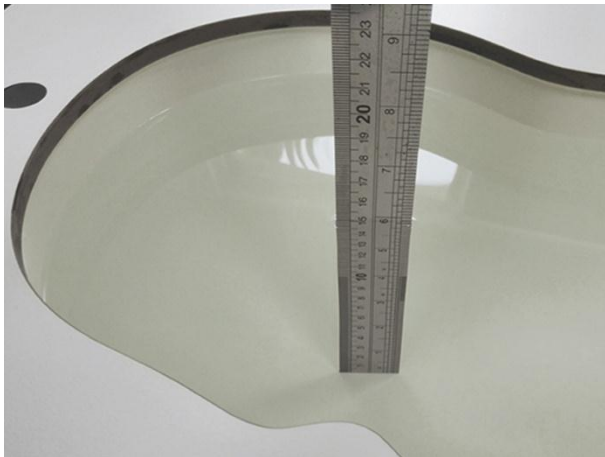
Liquid depth in the head phantom (2450MHz)
