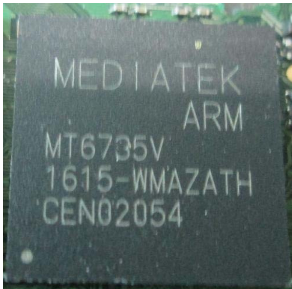
EUT – IC Chip View
