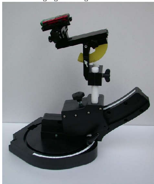
Device holder supplied by SPEAG
