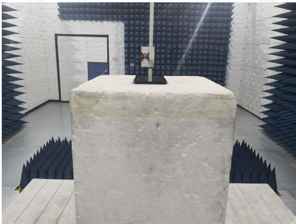
RADIATED EMISSION TEST SETUP ABOVE 1GHZ
