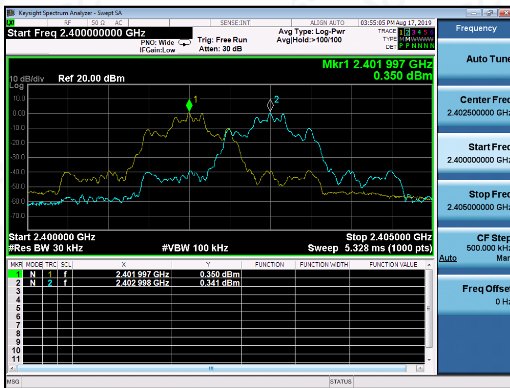
TEST PLOT FOR FREQUENCY SEPARATION
