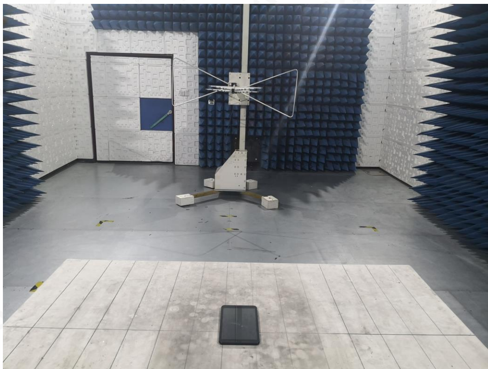
RADIATED EMISSION TEST SETUP ABOVE 1GHZ
