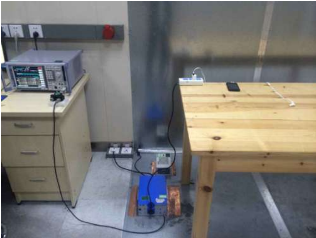
FCC RADIATED EMISSION TEST SETUP
