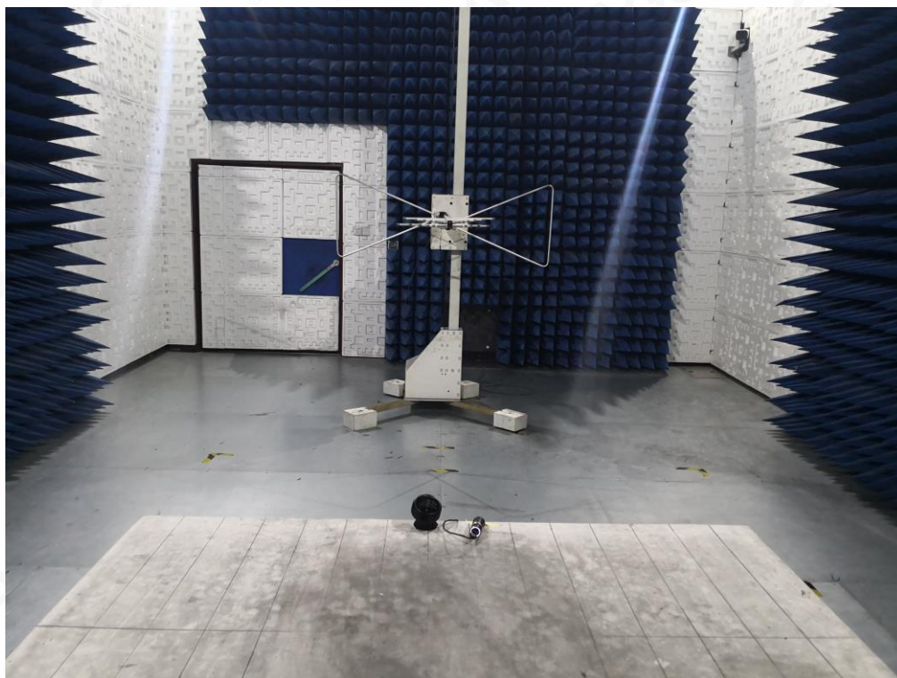
FCC RADIATED EMISSION TEST SETUP ABOVE 1GHZ
