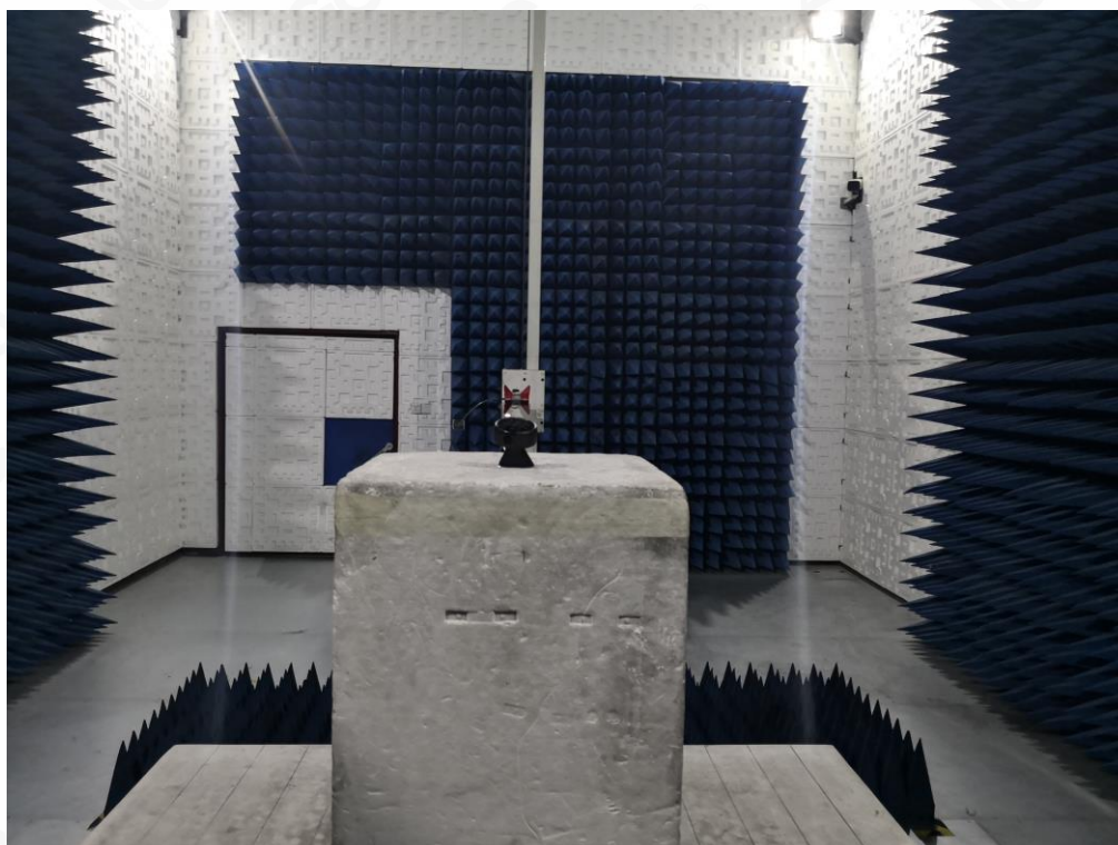
FCC RADIATED EMISSION TEST SETUP ABOVE 1GHZ
