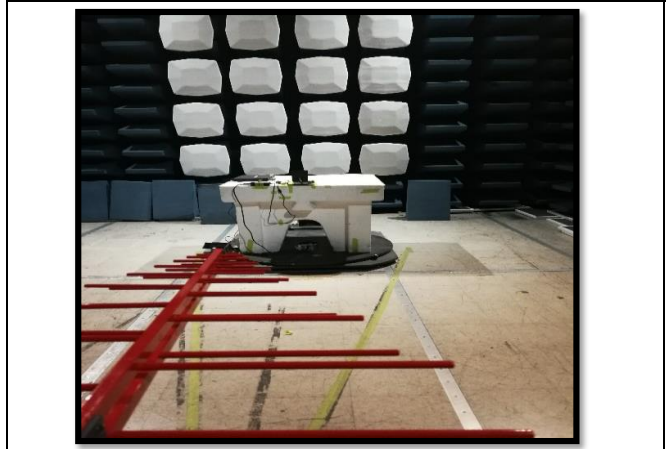
Figure R4: Radiated Emissions 30M-1G Test Setup
