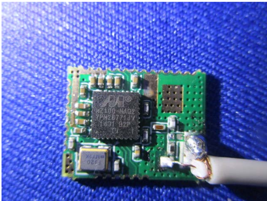
EUT- RF Chip View
