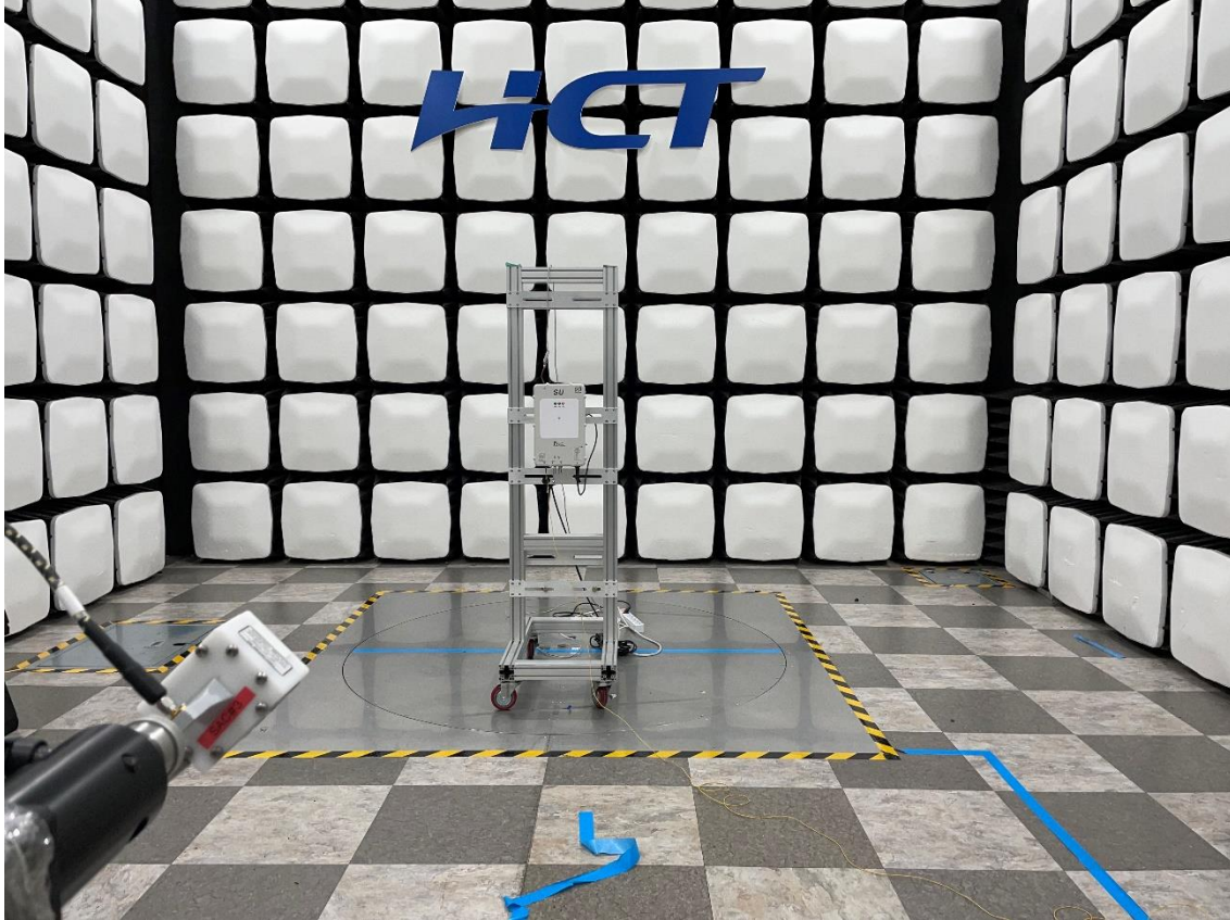
Radiated Test Setup Photo –Spurious (Horn Antenna 18 GHz ~ 40 GHz, 135°)
