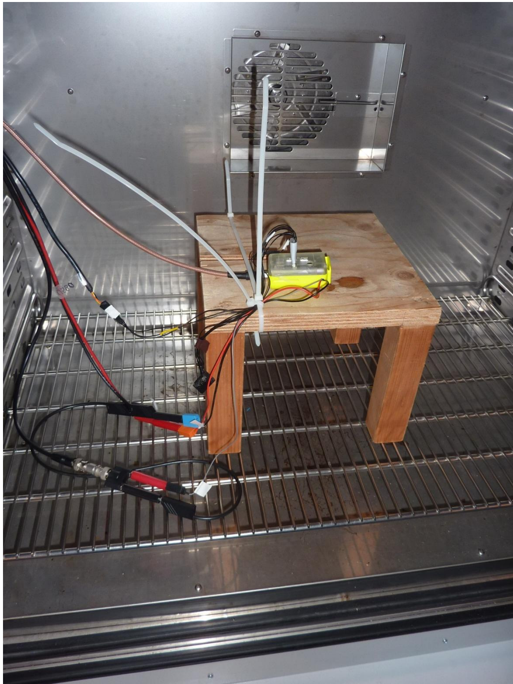
153662_5.JPG: SEAANGEL SA15 AIS FLARE, test set-up temperature chamber
