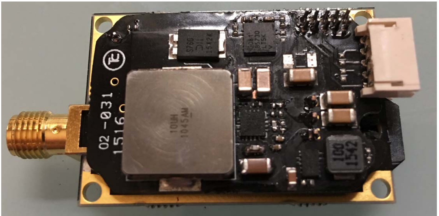
Power Supply Board, Side 1 (Note that RF board is attached under the power board in this photo.)
