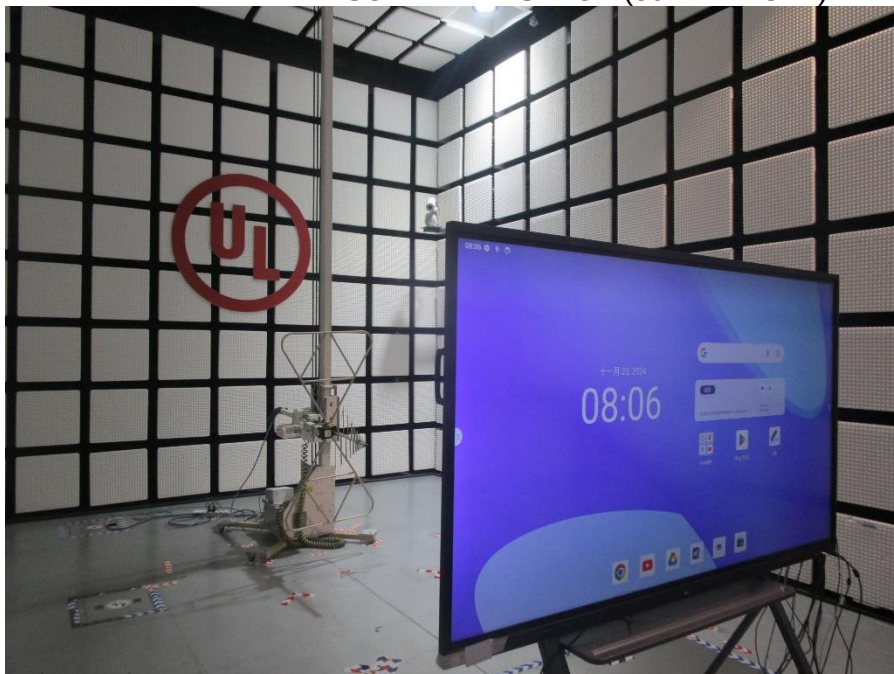
RADIATED RF MEASUREMENT SETUP (30MHz~1GHz)
