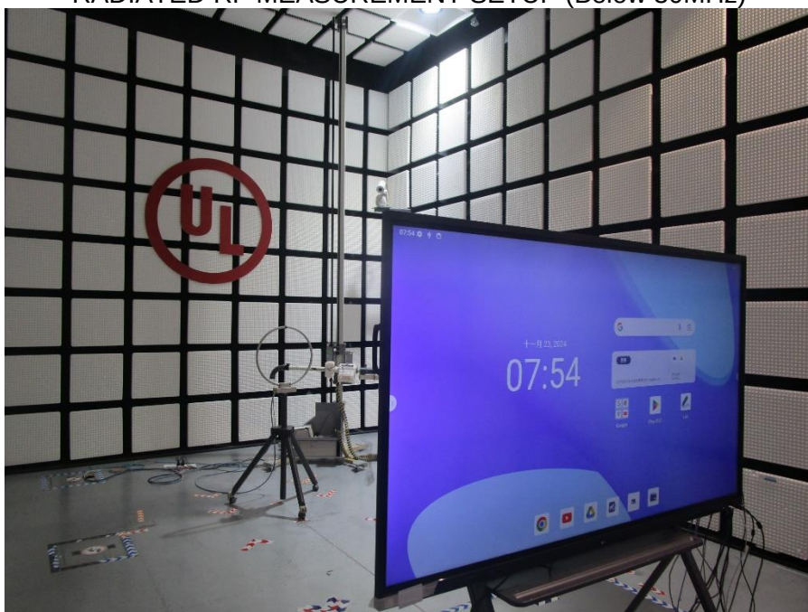
RADIATED RF MEASUREMENT SETUP (Below 30MHz)
