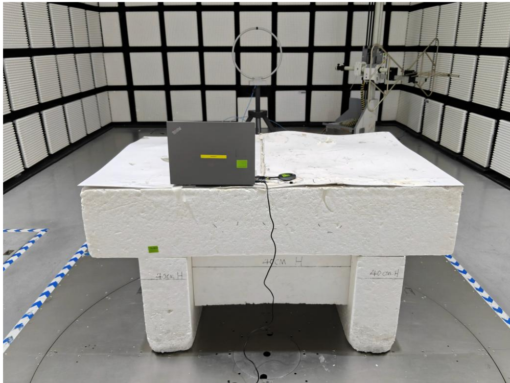
RADIATED RF MEASUREMENT SETUP (Below 30MHz)
