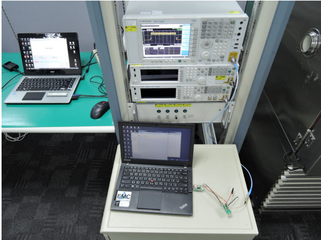
Photograph 4: Set-up for Conducted testing
