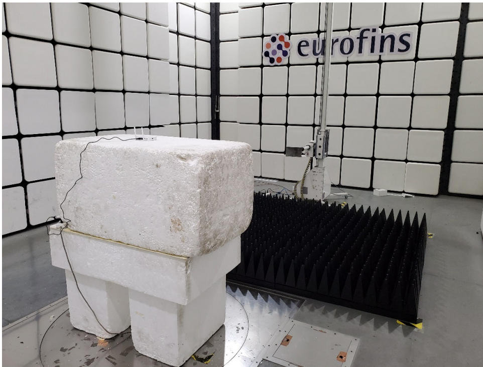
Picture 1 Radiated Emission Test Setup
