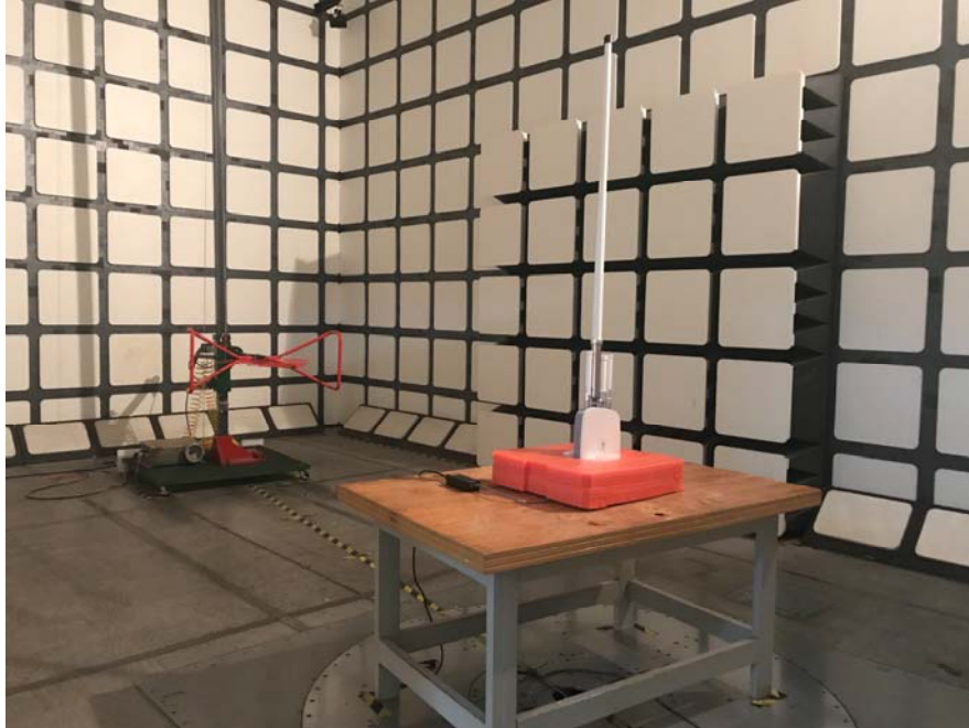
Radiated Emissions View (Below 1 GHz)
