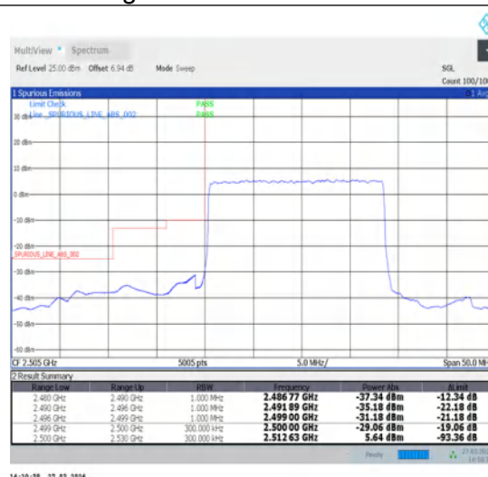
1-N7-15-20-L-3-DFT-PI2BPSK-Outer_Full-100@0-Ant1-1--PASS-see graph
