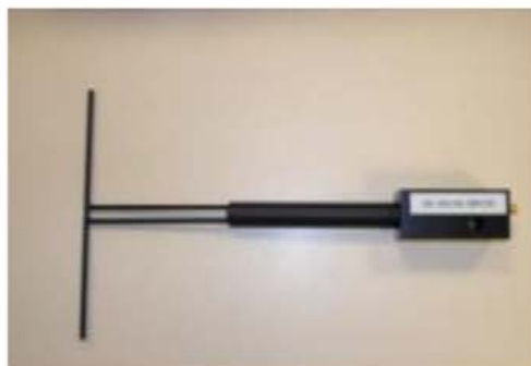
Figure 1 – Satimo COMOSAR Validation Dipole
