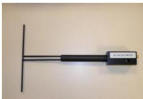
Figure 1 – Satimo COMOSAR Validation Dipole
