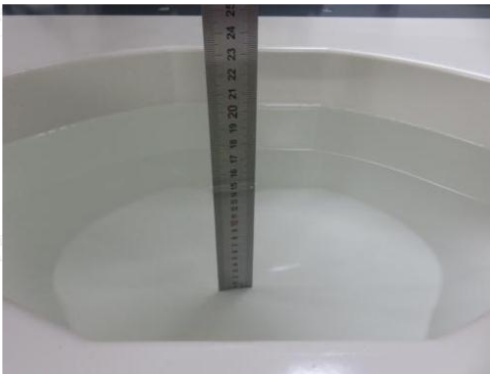
Photograph of the depth in the Body Phantom (2600MHz, 15.5cm depth)
