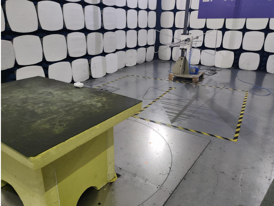
Spurious Emission Test Setup (Above 1GHz)
