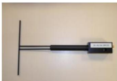
Figure 1 – Satimo COMOSAR Validation Dipole
