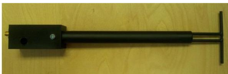
Figure 1 – MVG COMOSAR Validation Dipole
