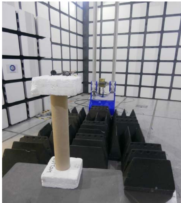
Radiated Emissions 1 GHz to 18 GHz
