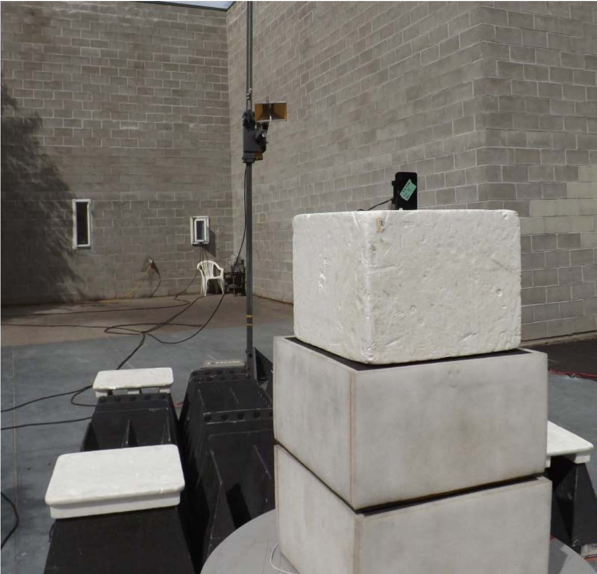
Figure E23.3 – Setup, Radiated Measurements 1 – 18GHz
