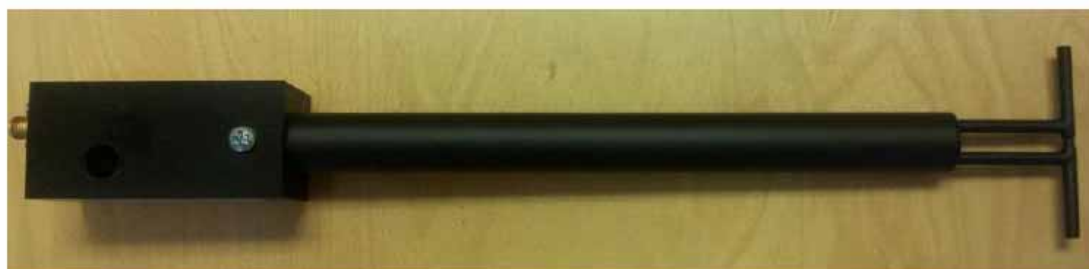
Figure 1 – MVG COMOSAR Validation Dipole
