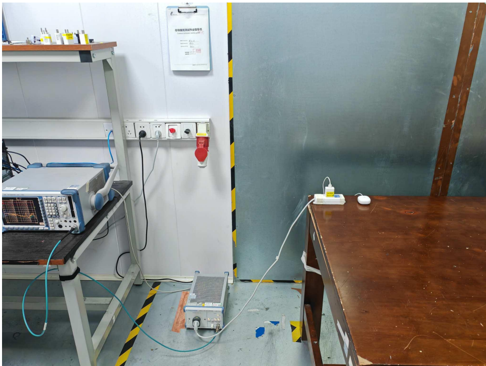
Conducted emissions at AC power line (150kHz-30MHz)
