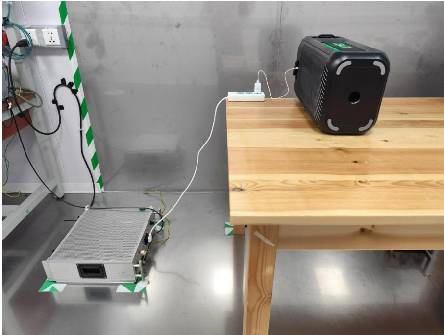
Conducted Emission at AC power line
