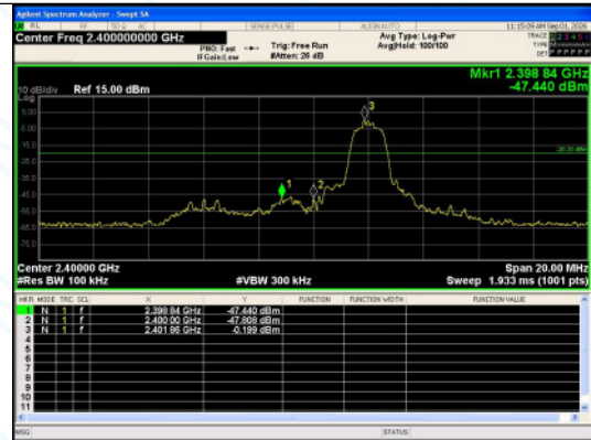
Out Of Band Emission \pi/4 DQPSK 2-DH5 Channel 0
