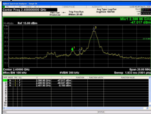
Out Of Band Emission GFSK DH5 Channel 0
