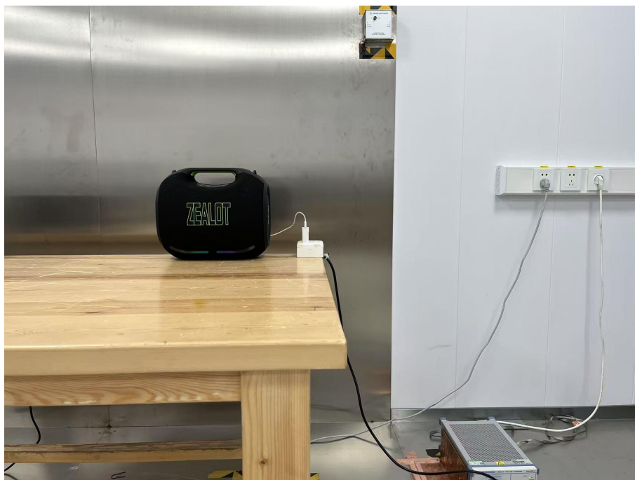
Radiated Emission Test View|(Below 1G)
