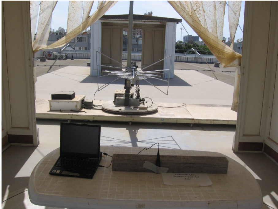
Figure 5. Radiated Emission Test
