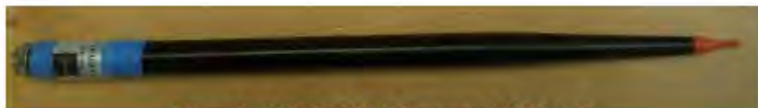
Figure 1 – MVG COMOSAR Dosimetric E field Dipole
