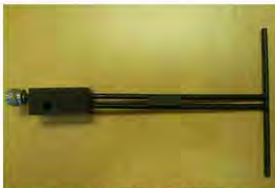
Figure 1 – MVG COMOSAR Validation Dipole
