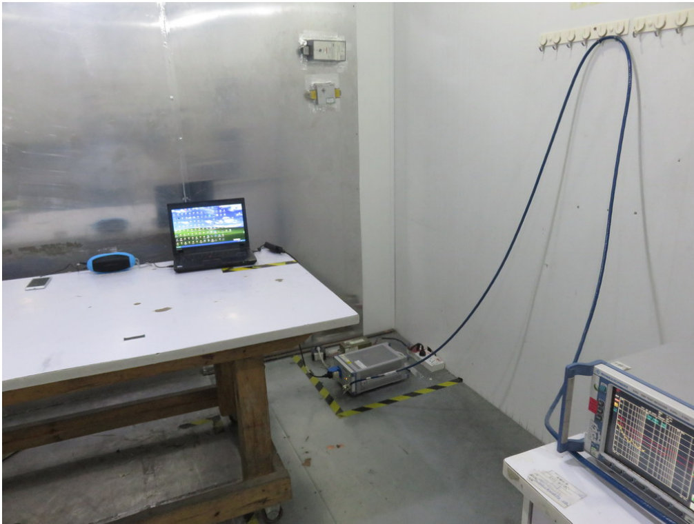
FCC RADIATED EMISSION TEST SETUP
