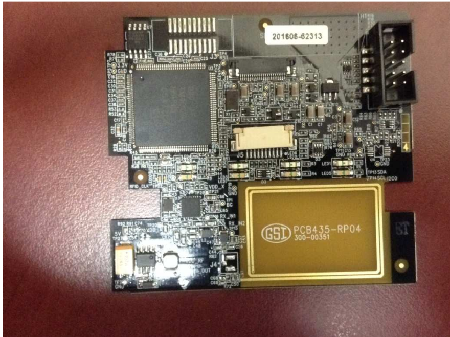
Top PCB of KP-8IN-1REL-components side
