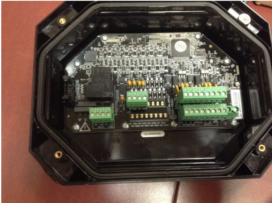
Bottom PCB of TR-2IN-1REL- components side
