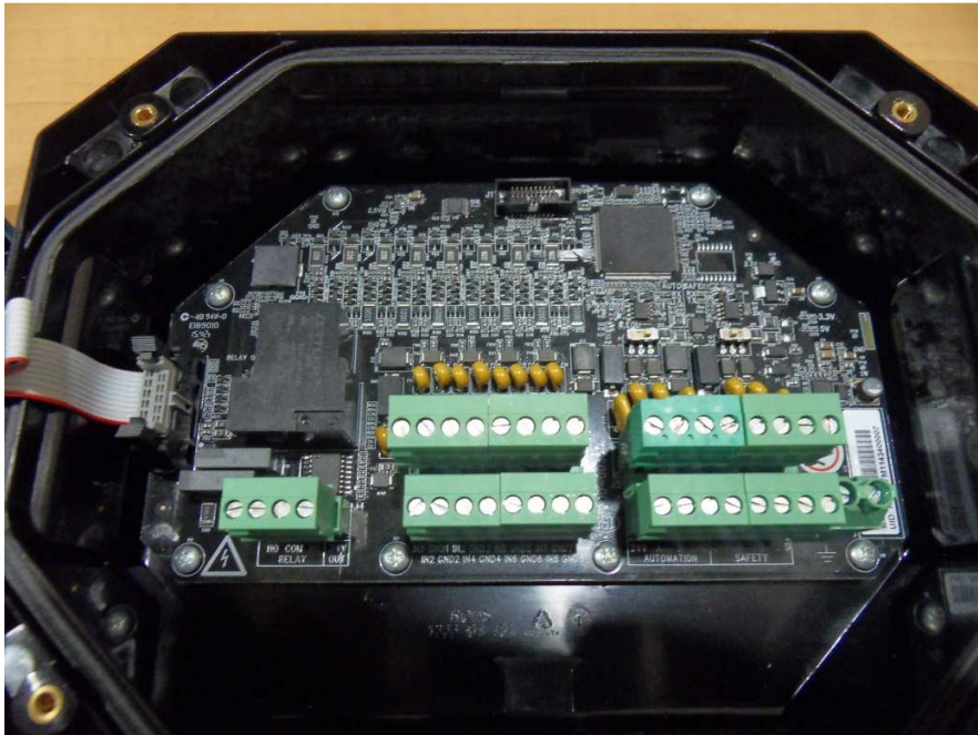
Bottom PCB of the KP-8IN-1REL – components side
