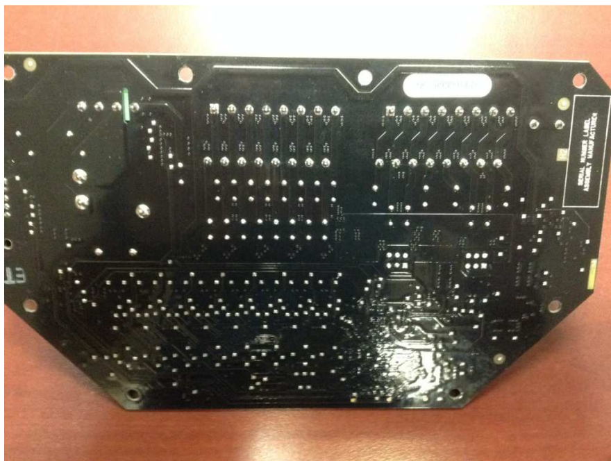
Bottom PCB of the KP-8IN-1REL – solders side
