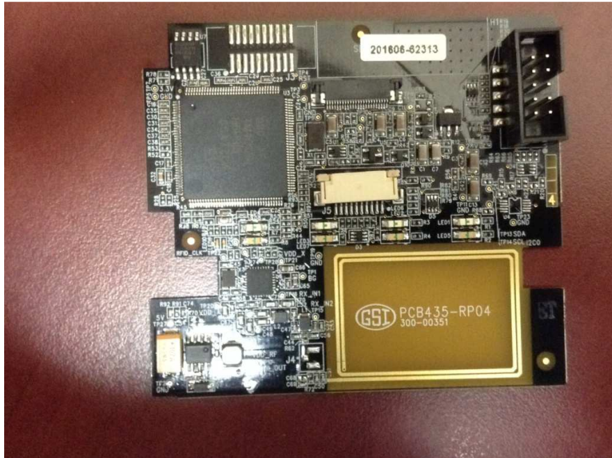
Top PCB of TR-2IN-1REL-components side
