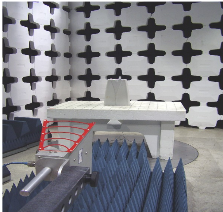
Photo 2. Radiated emission test setup
